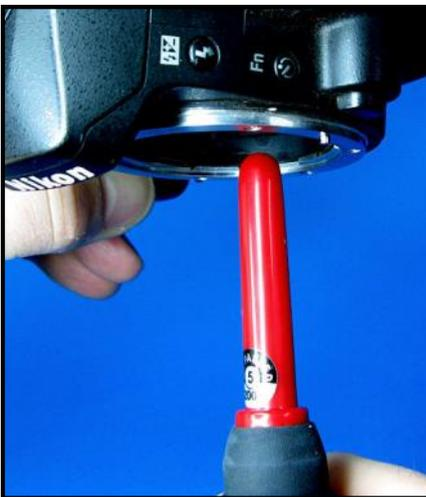
**Hold the camera with the lens opening downwards** and shake out anything that will come out that way. The use of a fine haired brush will help dislodge and clear other bits. Finally use your air puffer and gently puff out any remaining loose bits while holding the lens opening downwards.
